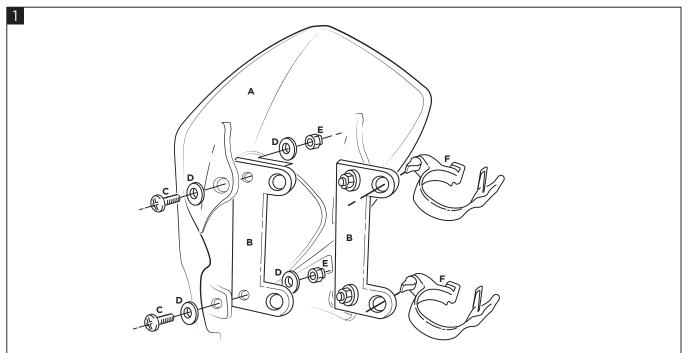
How to mount the headlight using the spacer plates provided in the mounting kit: Apply the spacer plates (B) to the headlight using the screws (C), the washers (D), and the nuts (E) provided in the kit. Fasten the plates (B) to the moto using the bands (F) as illustrated in the figure.
